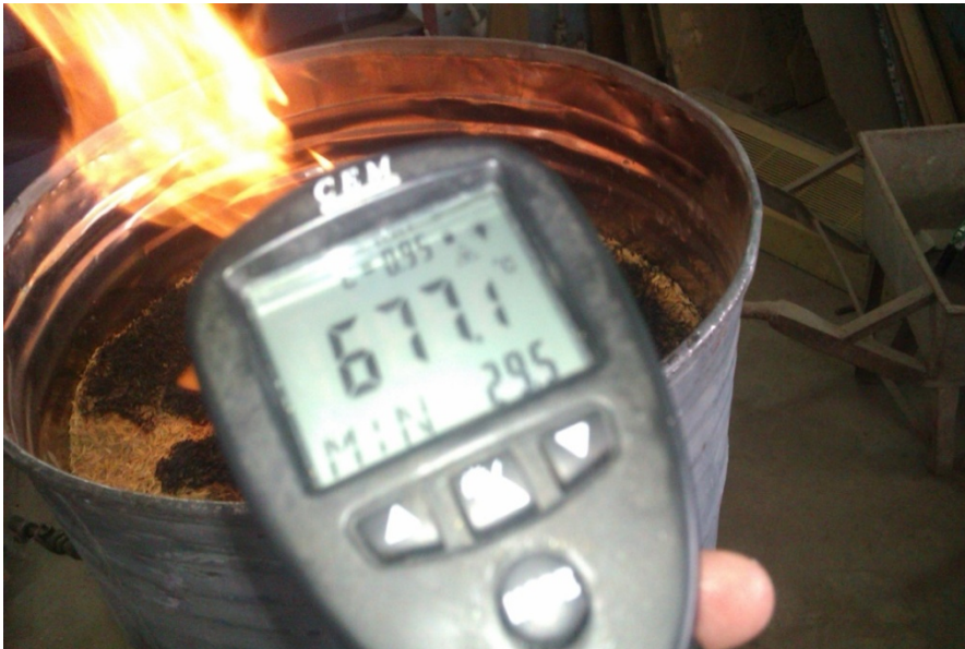
Figure 3. Burning of rice husk in a drum like kiln
